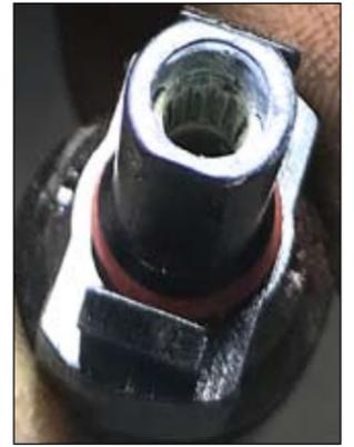
Corrosion inside the sealed MC4 plug and socket
