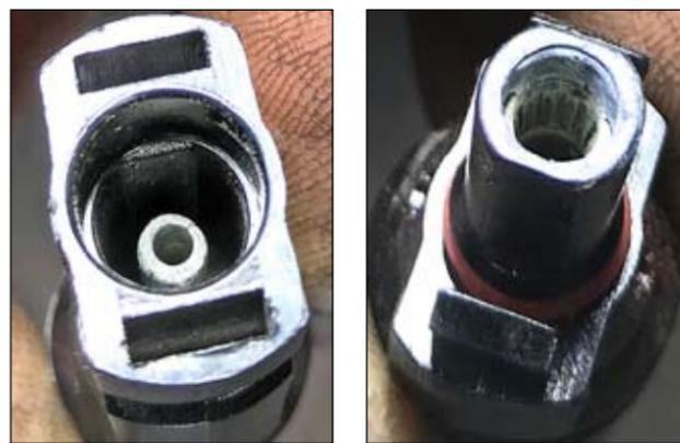
Corrosion inside the sealed MC4 plug and socket
