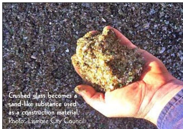
Crushed glass becomes a sand-like substance used as a construction material. Photo: Lismore City Council
